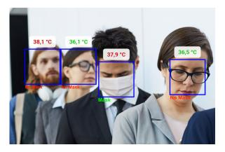
**Face-Mask Detection Platform** uses Artificial Network to recognize if a user is not wearing a mask. The app can be connected to any existing or new IP cameras to detect people without a mask. If the camera captures an unrecognized face, a notification can be sent out to the administrator.
